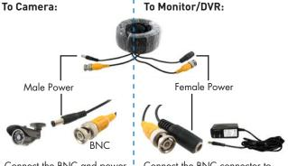
Connect the BNC and power connectors to the camera
